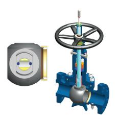
3. When the core has turned 90° the stem stops rotating and continues to lower with its linear movement. During the rotation, the core does not come in contact with the seat.
