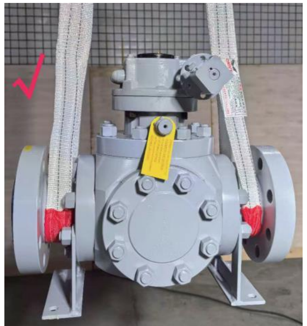
Figure 1-A Correct Valve Handling
